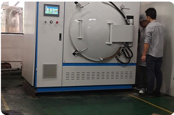
Integrated Experimental Furnace for Carbonization and Graphitization of Carbon Paper / Carbon Cloth for Fuel Cells image 4
