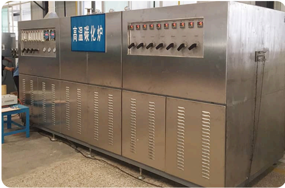
Continuous Carbon Fiber Carbonization Furnace image 2
